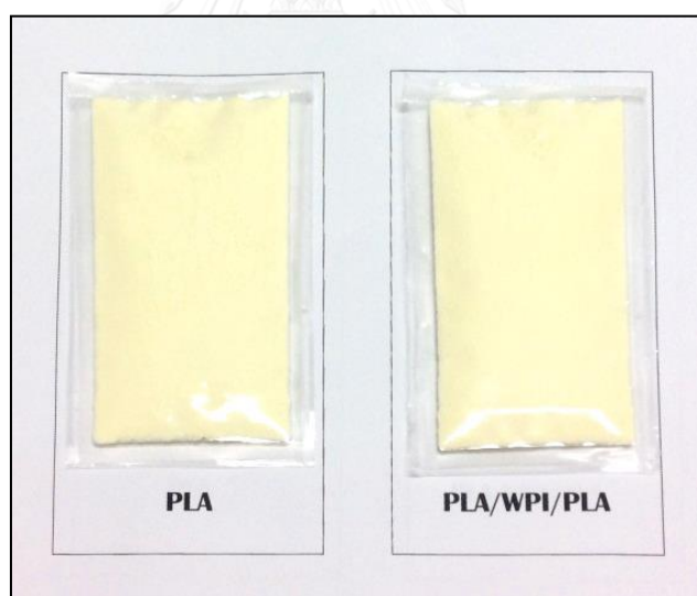
Figure 4.13: Baby formula packed in polylactic acid (PLA) and whey protein isolated (WPI)-enhanced composite structures (PLA/WPI/PLA) four-side-seal pouches.
