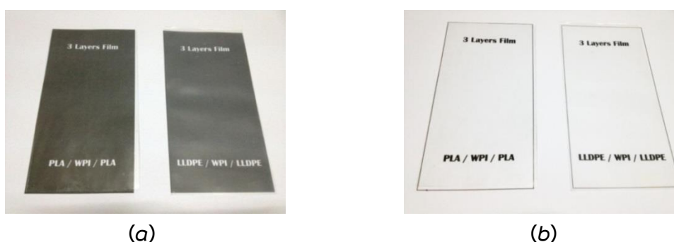
Figure 4.1: Multi-layer structures made of glycerol-plasticized whey protein isolate (WPI) sandwiched between two substrates, polylactic acid (PLA) and linear low-density polyethylene (LLDPE). PLA/WPI/PLA and LLDPE/WPI/LLDPE film samples were displayed on a dark (a) and a white (b) background.
