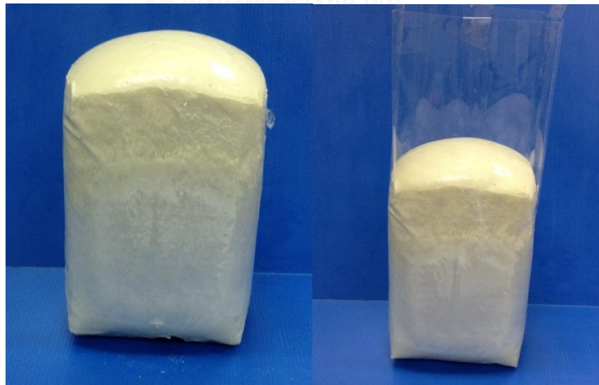
Figure 4.12 RPUR foam prepared by using a plastic bag
