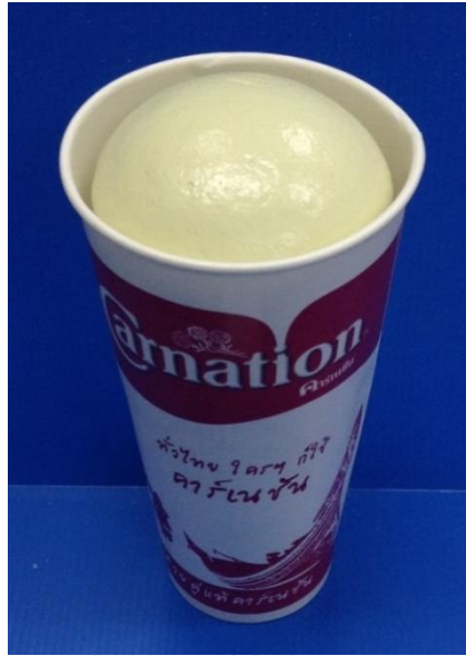
Figure 4.11 RPUR foam prepared by using a 700 ml paper cup
