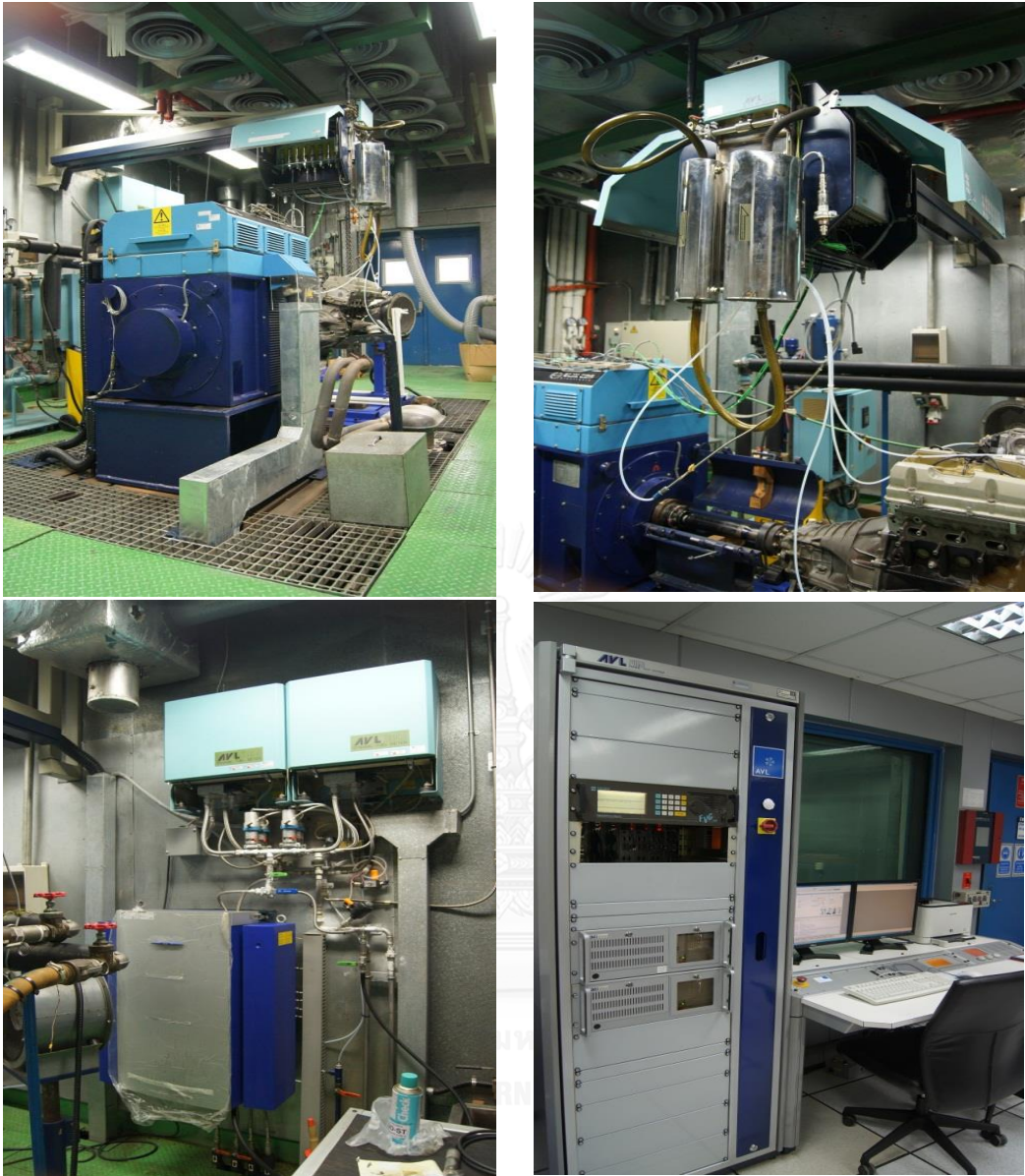
Figure 17: Automated engine test system for engine combustion analysis
