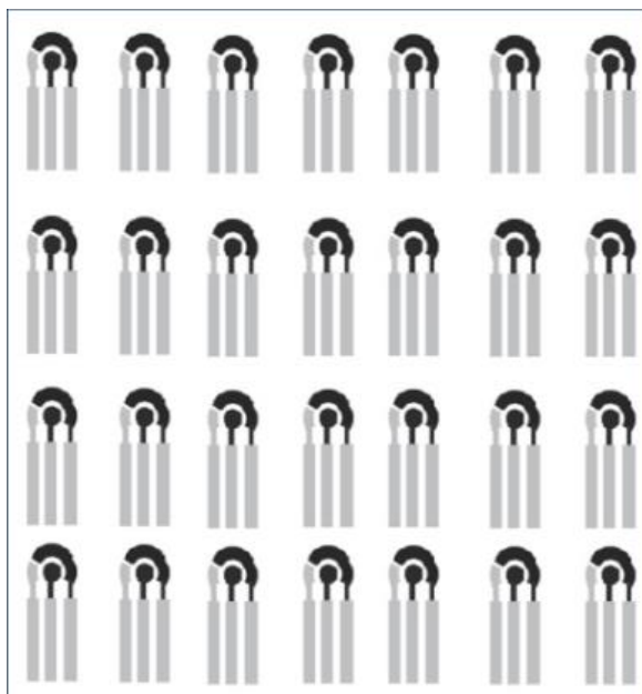
Figure 3.1 Screen-printed carbon electrodes using a manual screen-printing technique.
