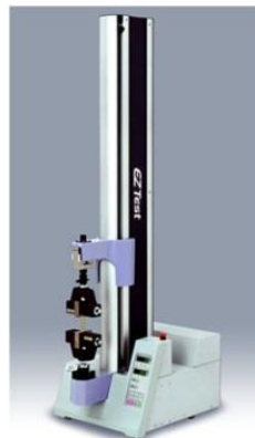
Universal testing machine (Shimadzu Corp., Japan) for shear bond strength test
