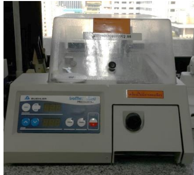
Low speed cutting machine (ISOMET 1000, Buchler, USA)
