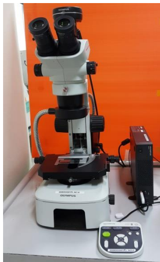
Stereo microscope (SZ61 Series, Olympus,) for evaluation of the residual adhesive
