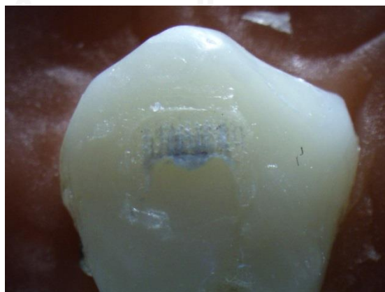
Figure 14 Scale 3 indicates that more than 10% but less than 90% of the adhesive remained on the tooth surface
