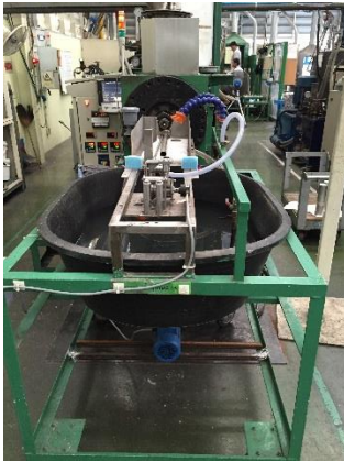
Figure 3. 4 Extrusion machine used for production of water soluble rosin flux cored solder wire.
