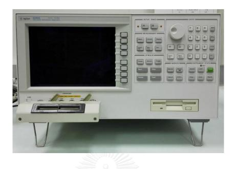
Figure 4.13: Impedance analyzer (Agilent 4294A).
