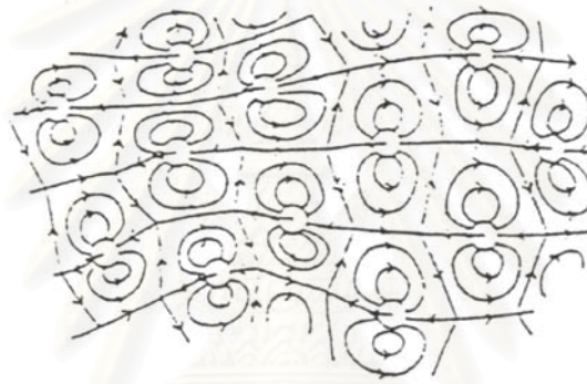
Figure 3.1b Mean flow velocity around cylinder
