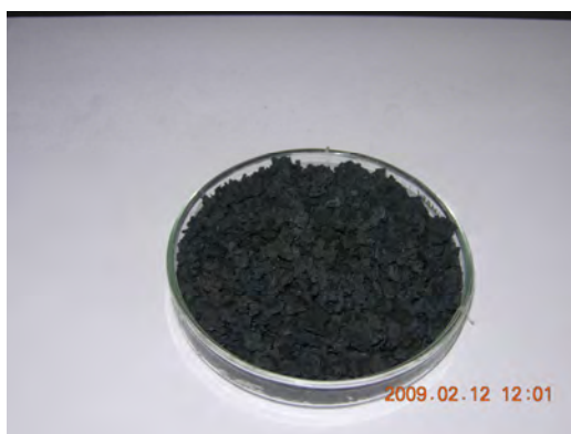
Figure 4.8 sludge char before activation.
