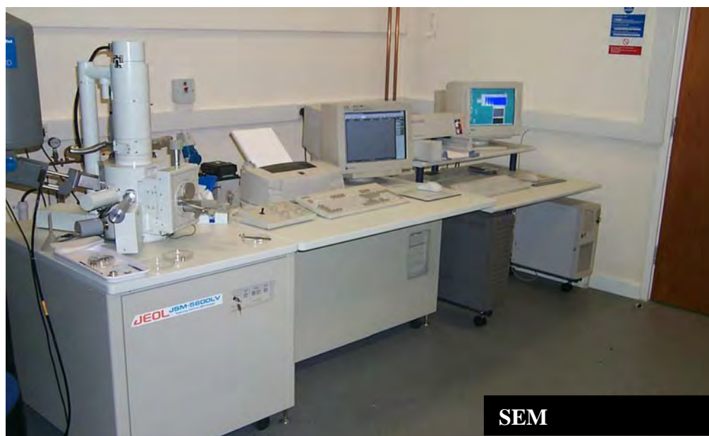
Figure 5.19 Photograph of an SEM (at School of Chemistry, University of Bristol).
