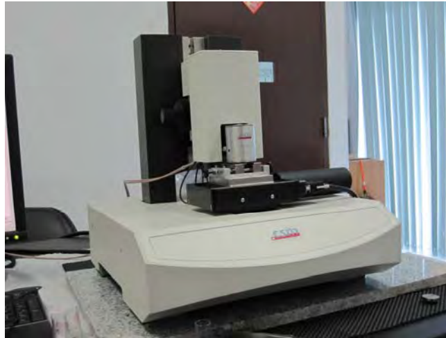
Figure 5.23 Photograph of Nanoindentation apparatus (at Nano shield co., Ltd, Thailand).
