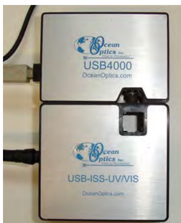
Figure 5.11 Photograph of the UV-VIS spectroscopic holder (at School of Chemistry, University of Bristol).
