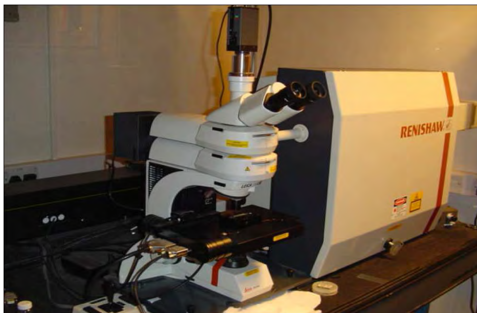
Figure 5.2 Photograph of the Renishaw 2000 LRS microscope (at School of Chemistry, University of Bristol).
