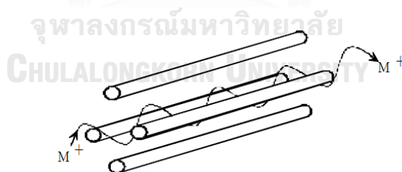
Figure 2.14 Quadrupole Mass Analyzer [53].
