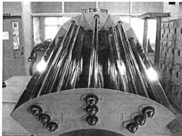
Figure 10. The second prototype of parabolic trough solar collector with no need of solar tracking system which has an overall width of 0.7 m and a length of 1.4 m.
