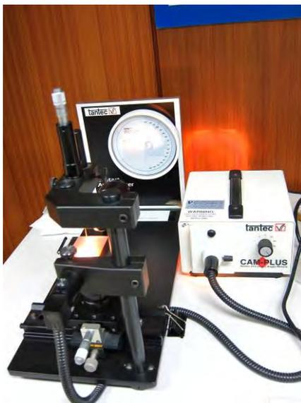
Figure 3.9 CAM-PLUS Tentec contact angle meter
