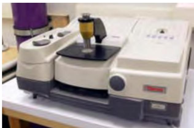
**Figure 3.8** Nicolet6700 Fourier-Transformed Infrared Spectrophotometer
