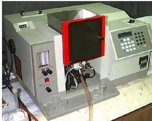
Figure 3.6 AAS model SpectrAA-300 atomic absorption spectrometer.
