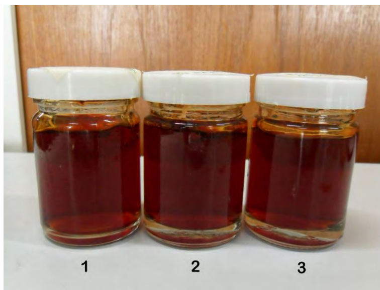
Figure 16. An appearance of TSCE gel: After freshly prepared (1); After stored at room temperature for 12 wks (2); and After freeze-thaw cycle for 3 cycles (3).
