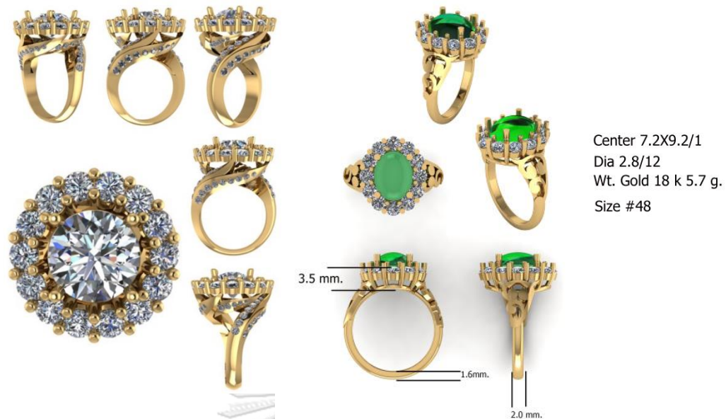
Figure 25: Realistic 3D Rendering to Show Customer Design Prototypes
