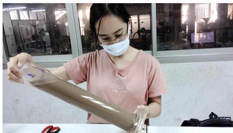
Figure 3.10 The agitation of the slurry for a period of 1 min
