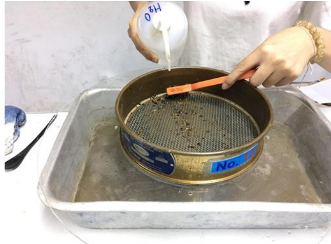
Figure 3.8 Separate particle size larger No. 10 (2 mm)
