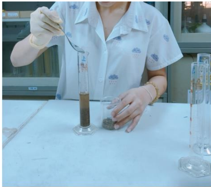
Figure 3.16 Put the sample in the graduate cylinder
