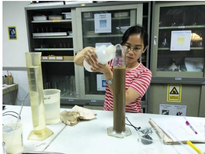
Figure 3.9 Preparing the suspension for hydrometer test
