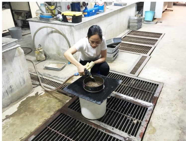
Figure 3.11 Making a wet sieve analysis
