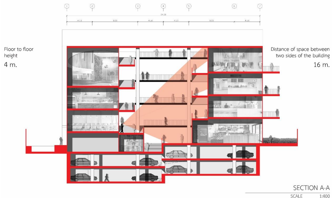
Figure 5.13 The section of the proposed community mall with visible parts from the first floor highlighted in red.
