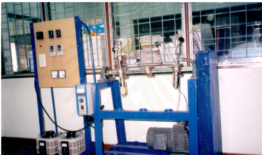
Figure 4.1 The Reaction Experimental Unit for conversion of polyethylene into gasoline using HZSM-5 type catalyst.
