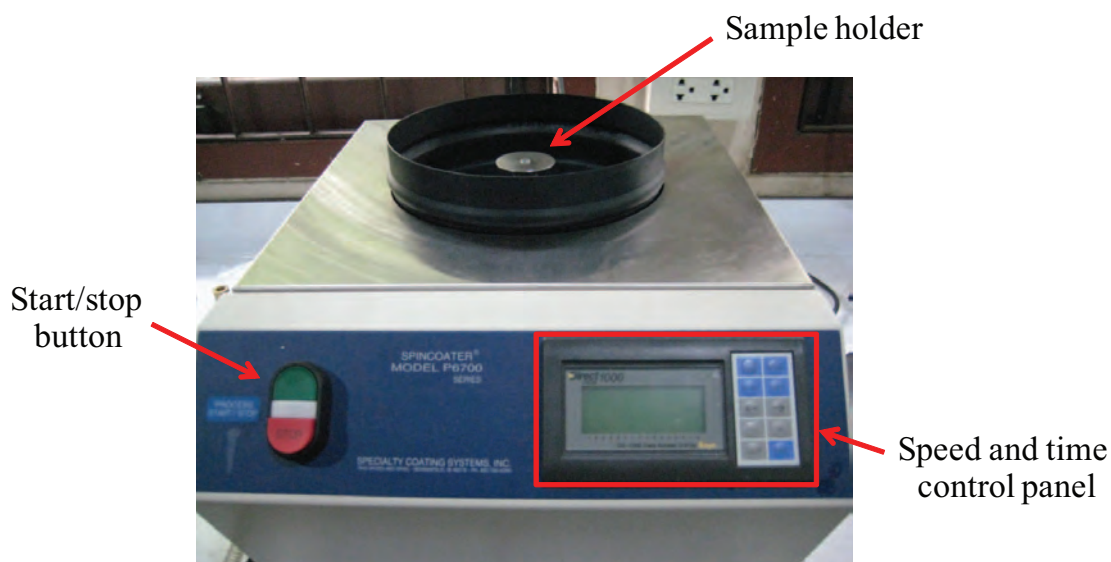
Figure 4.2: Spin coater (SPIN COATER model P6700 series).
