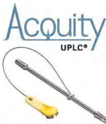
Figure 2.2 Illustration of UPLC column with eCord™ [39]
