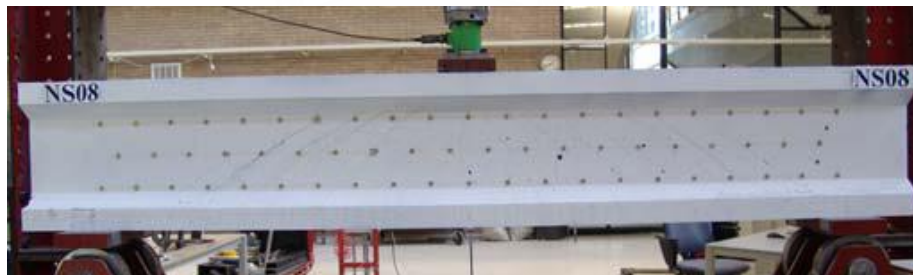
Figure 4.6: Test set up for I-beam failed by shear
