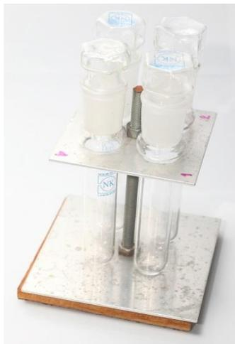
**Figure 2.21** Custom-made quartz tubes and their stand
