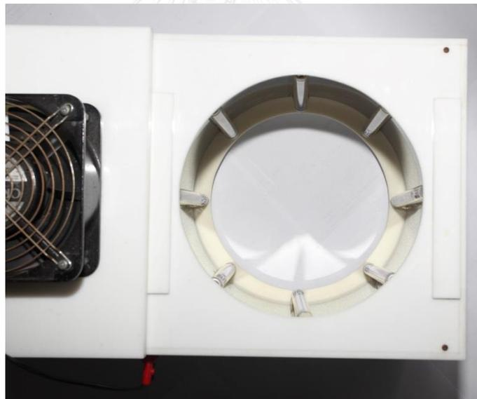
Figure 2.20 Home-made UV reactor showing UV lamps
