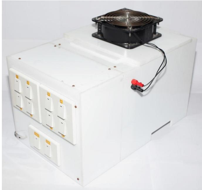
Figure 2.19 Home-made UV reactor
