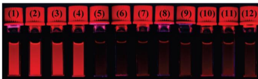
Figure 2.4 Photographs of the luminometric responses of the \text{Ru}_2\text{Eu-1} ( 1.0 \times 10^{-4} M) in EtOH at 298 K: (1) \text{Ru}_2\text{Eu-1} + histamine; (2) \text{Ru}_2\text{Eu-1} + putrescine; (3) \text{Ru}_2\text{Eu-1} + spermidine; (4) \text{Ru}_2\text{Eu-1} + \text{NH}_3 ; (5) \text{Ru}_2\text{Eu-1} only; (6) \text{Ru}_2\text{Eu-1} + aniline; (7-12) \text{Ru}_2\text{Eu-1} + \text{H}_2\text{S} , CO, \text{N}_2 , \text{CH}_4 , \text{H}_2 , and air, respectively. (1) Excitation \lambda_{\text{ex}} = 365 nm [35]
