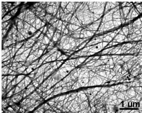
Figure 2.6 Transmission electron micrographs of microfibrillated cellulose [5].
