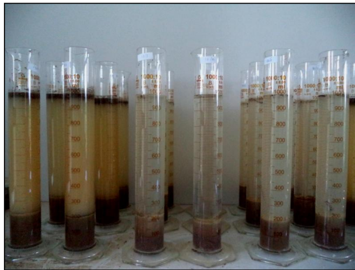
Figure 18 The settling of particles in soil suspension
