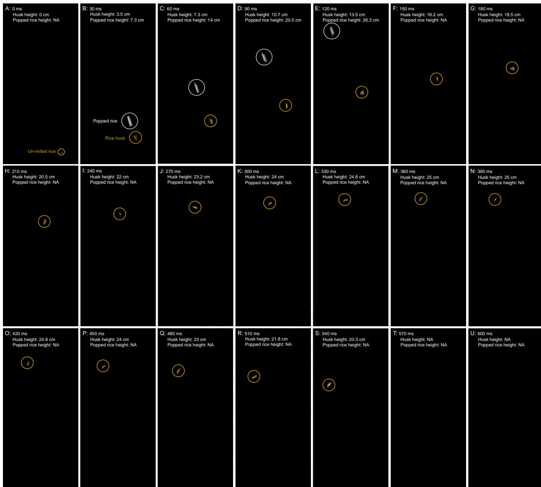
Figure 4.2 A series of still images with 30 ms interval extracting from a slow-motion VDO clip shows trajectory of popped rice and its husk as the grain popped upon heating. This particular rice grain popped at 209.5 °C as indicated by the thermocouple. With Photoshop software, the positions of popped rice and its husk were overlaid on the same image.
