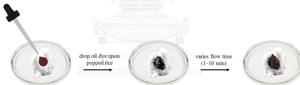
Figure 3.7 Schematic drawing of a drop of red organic dye on top of popped rice.
