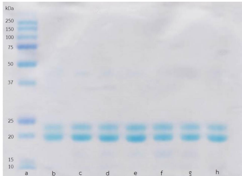
Figure 3 SDS-PAGE result; standard marker (a); commercial zein (b); zein extracted from CGM batch no. 150113 (c), 280813 (d), 241214 (e, g) using 70% v/v aqueous ethanol; zein extracted from CGM batch no. 241214 using 60% v/v (f) and 80% v/v (h) aqueous ethanol
