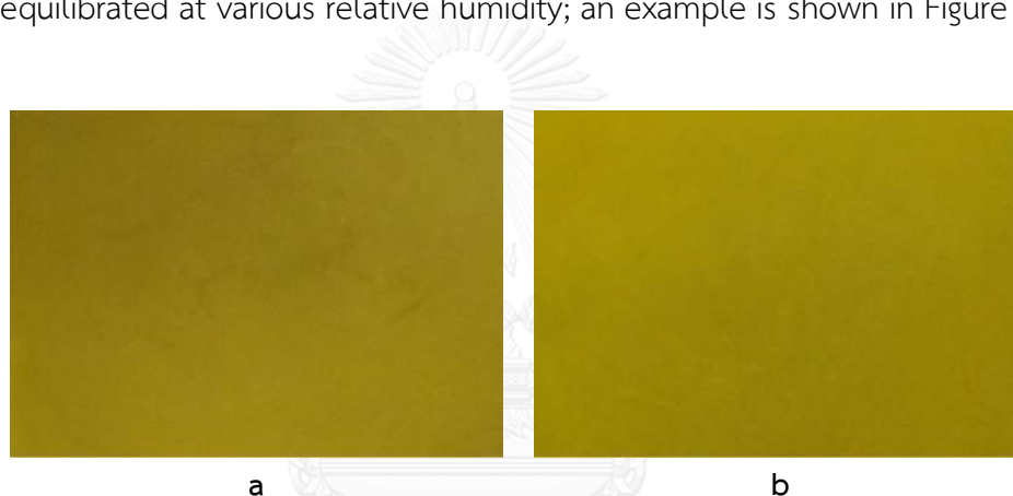
Figure 4 Photographs of CZ film; films prepared without glycerol equilibrated at 52% RH (a), and with glycerol equilibrated at 52% RH (b)
