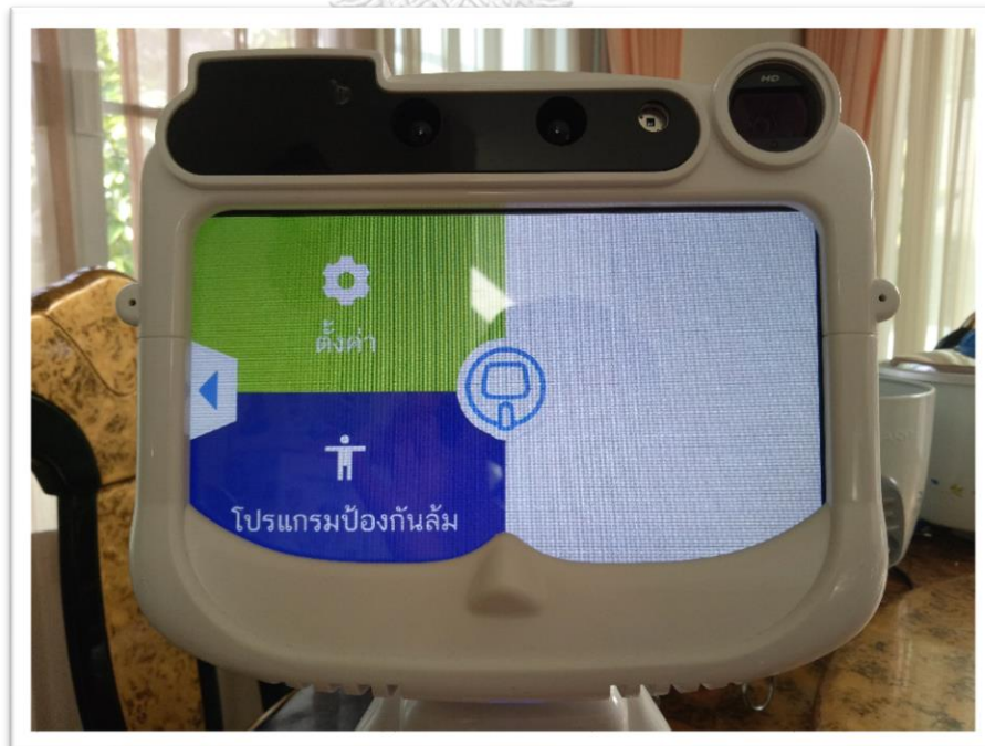
Figure 12 Fall prevention software installed in Dinsow Mini Robot®
