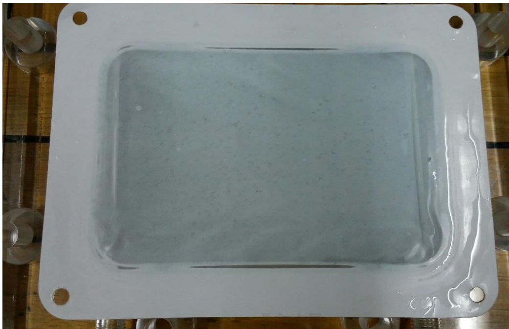
Figure 5.3 Condition of membrane sheet after treatment of wastewater
