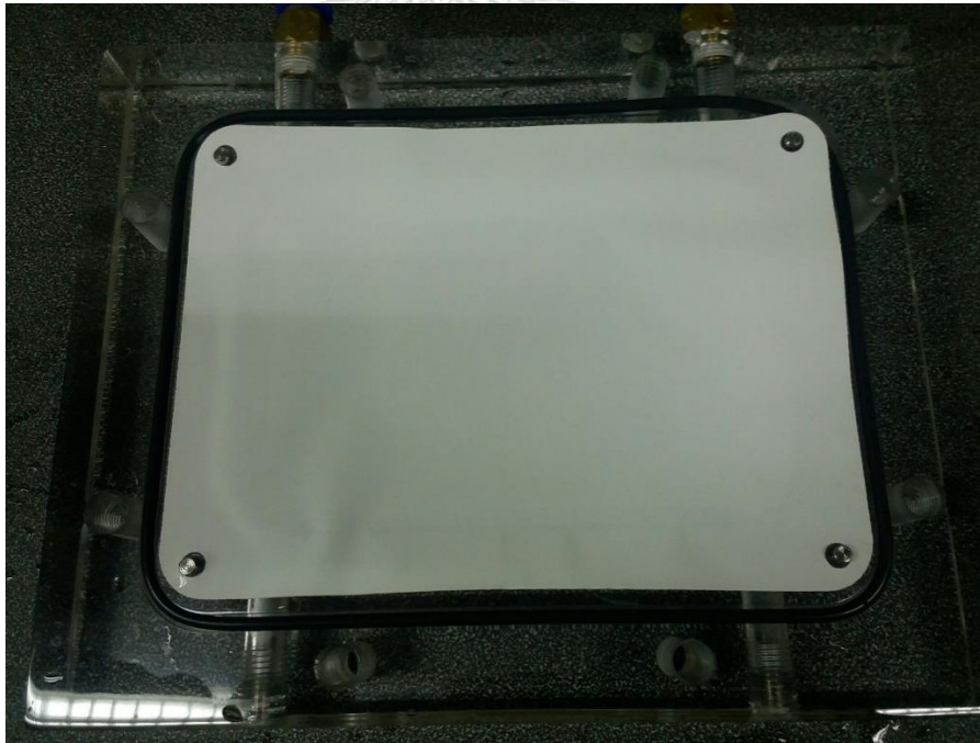
Figure 5.2 Virgin membrane flat sheet (PVDF)
