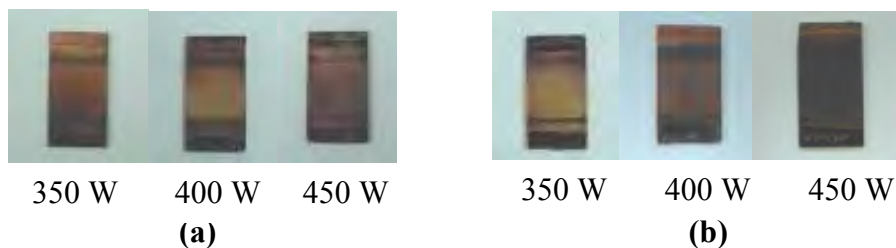
Figure 4.1 Examples of plasma-polymerized films by microwave plasma polymerization at different microwave power (a) poly(2-methylthiophene) and (b) poly(3-methylthiophene).
