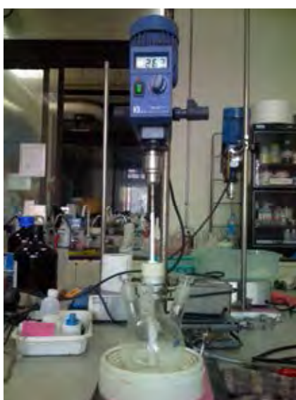
Figure 3.1 Apparatus for mesoporous rp-SBA-15 synthesis.
