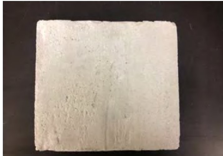
Figure 3.4 Typical concrete slab for laboratory- scale testing
