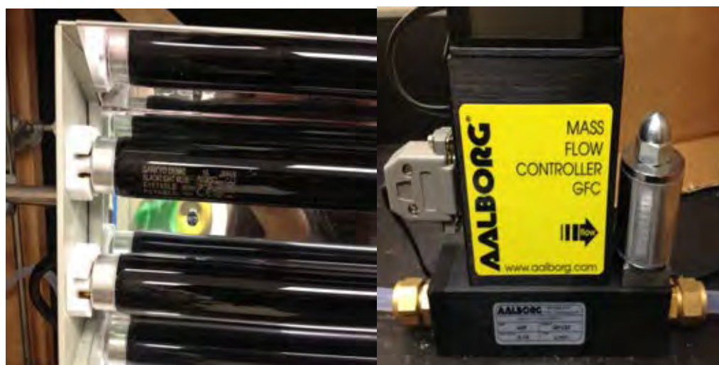
Figure 3.2 Mass flow controller and Black Light Blue (BLB) fluorescent lamps 15 W UV-A illumination
