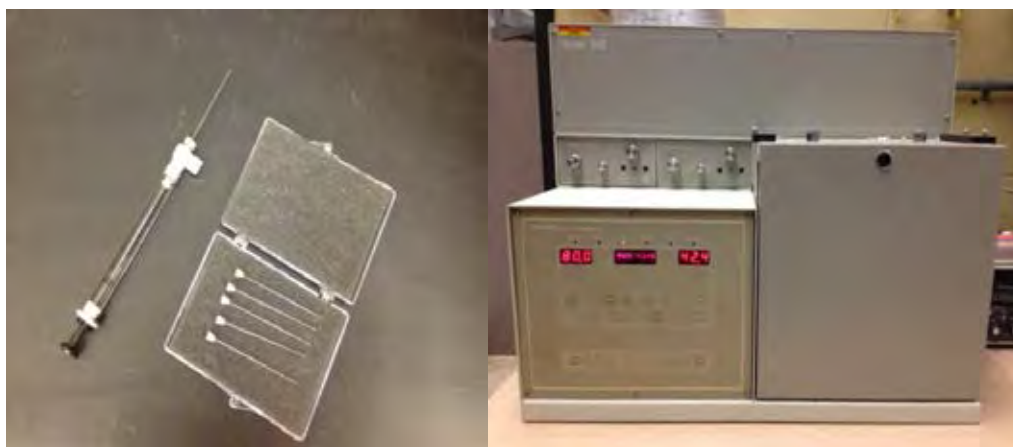
Figure 3.9 One mL syringe and Tracor 540 gas chromatograph
