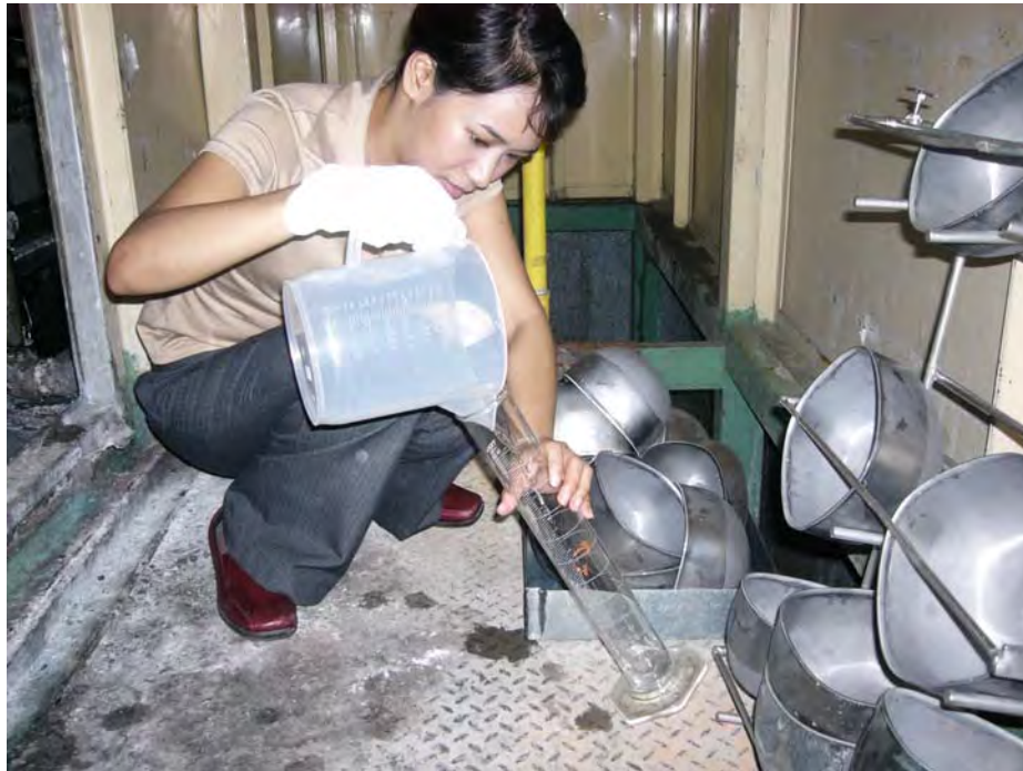
Figure 4.6 Measure drag out from rinsing.
