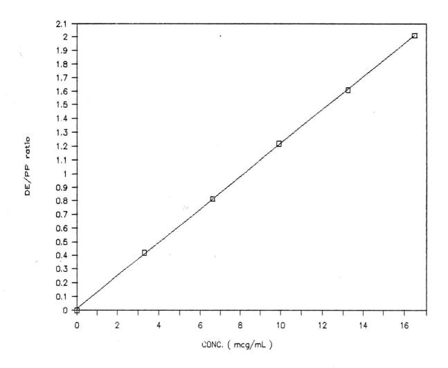
Figure 15 A HPLC calibration curve of DE solubility and stability study
