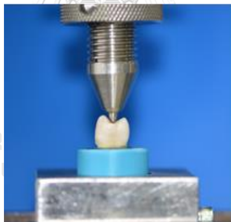
Figure 5 specimens were tested using a universal machine
