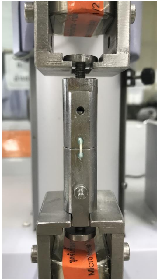
Figure 4 Microtensile bond strength testing
