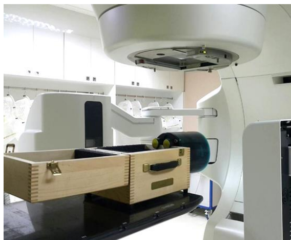
Figure 3.12 Catphan ® 600 phantom setup for linear accelerator
