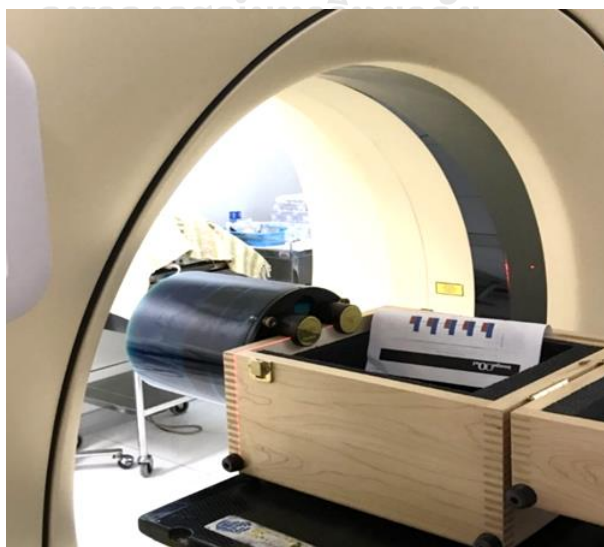
Figure 3.11 Catphan ® 600 phantom setup for CT simulator
