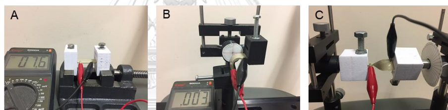
Figure 3.4 The mechanical strain devices (A) stretching, (B) bending, (C) twisting for electrical resistivity measurement.
