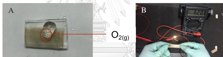
Figure 4.24 (A) Digital images of hydrogen peroxide testing, confirming that silver structures were adhered on PDMS surface after fabrication. (B) LED light testing while the two-point probe multimeter was clipped on the surface of a strip.
