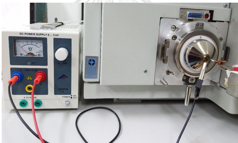
Figure 2.1 Experiment setup for paper spray mass spectrometry.
