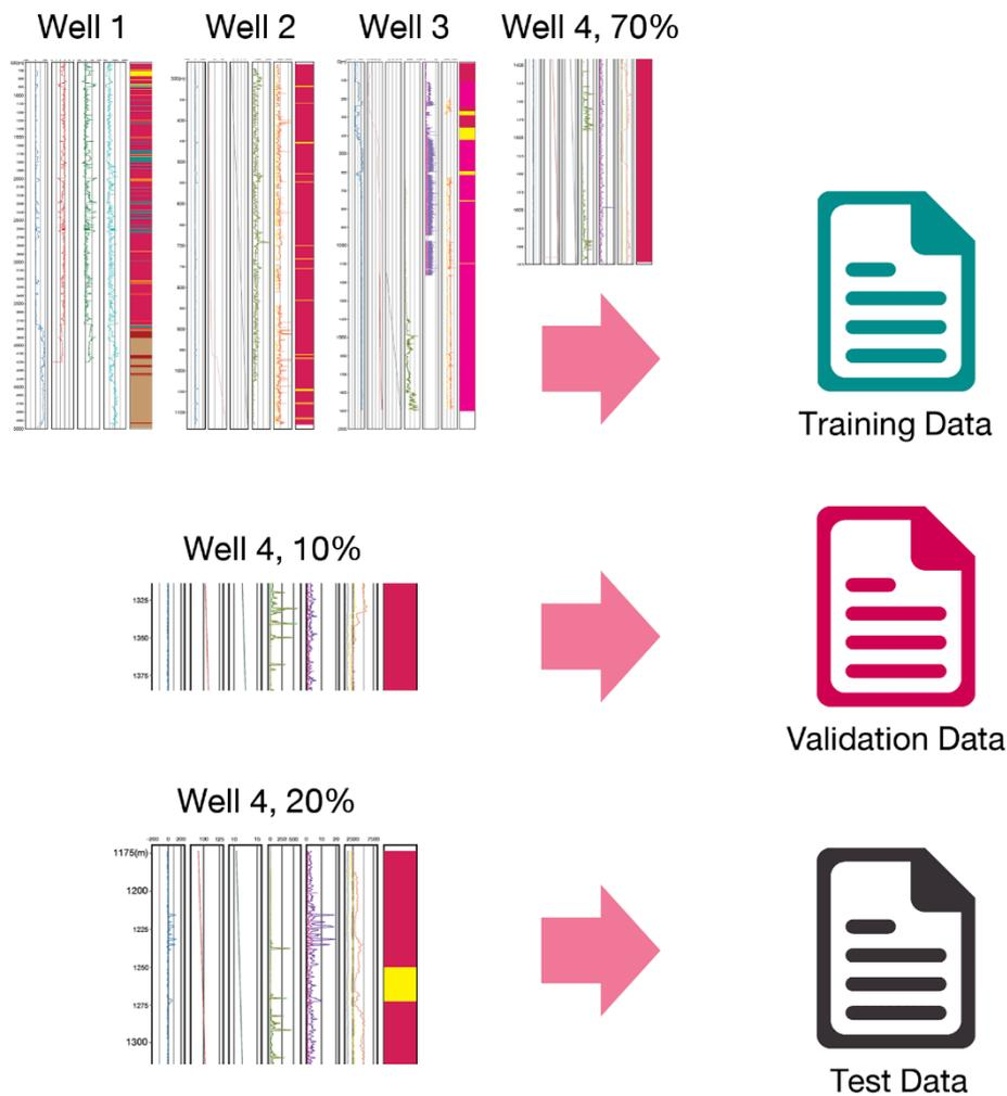
Figure 37 The multiple-well test. Three wells and 70% of the fourth well are assigned as training data while the rest of the fourth well is assigned as validation (10%) and test (20%) data.
