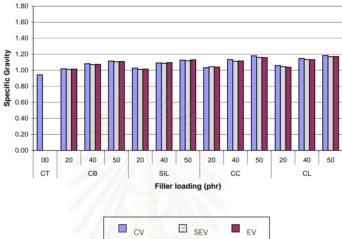
Figure 4.3 Effect of curing system, filler types and loading on specific gravity.
