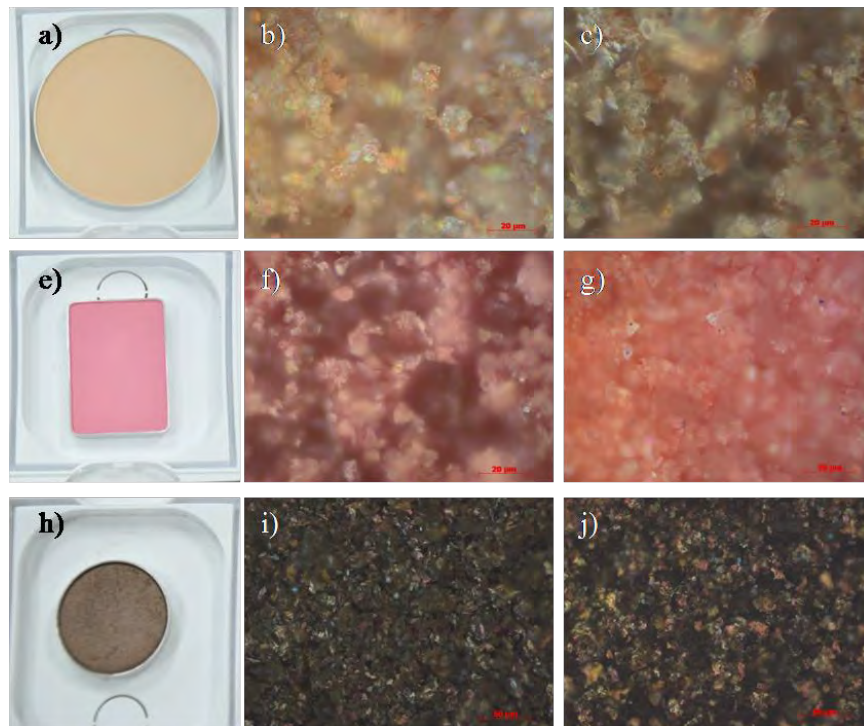
Figure 4.20 Photographs and optical microscope images of bright field and dark field of (a), (b), and (c) press powder, (e), (f), and (g) brush on, and (h), (i), and (j) eye shadow which were mixed pearlescent flakes from green mussel shell.
