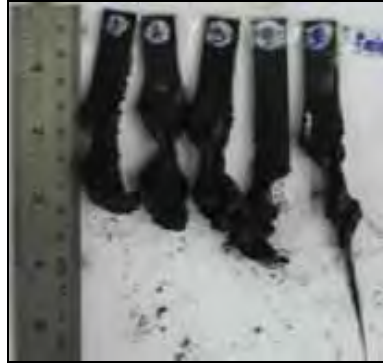
Figure 4.11 Sample specimens of PC11 according to UL94 5VB test.
