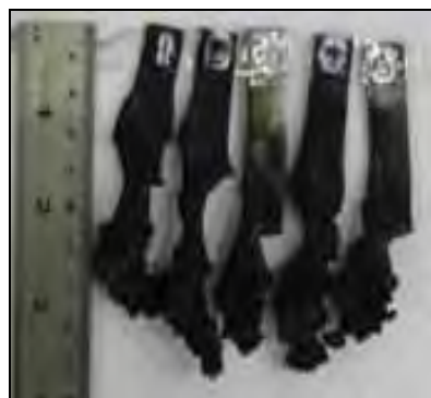
Figure 4.10 Sample specimens of PC10 according to UL94 5VB test.
