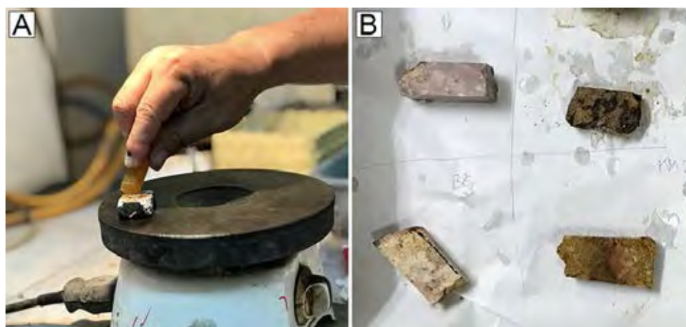
Fig. 3.8 Thin section preparation. A. Melted balsam put on the target side of rock slab, B. rock slabs.
