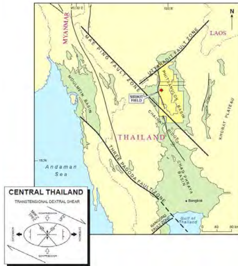
Figure 2.2 The Phitsanulok Basin associated with the Uttaradit and Mae Ping fault zones (Flint et al., 1988)
