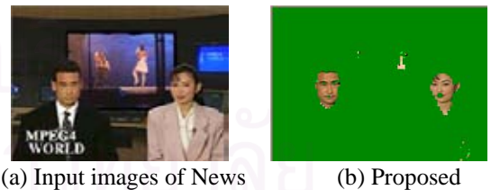
Figure 3. Result of proposed color components reference maps in YCbCr and HSV color space.
