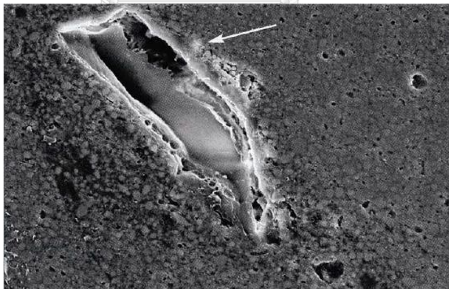
Figure 3 An electron microscope image showing a gap (50x10 microns) (27)
