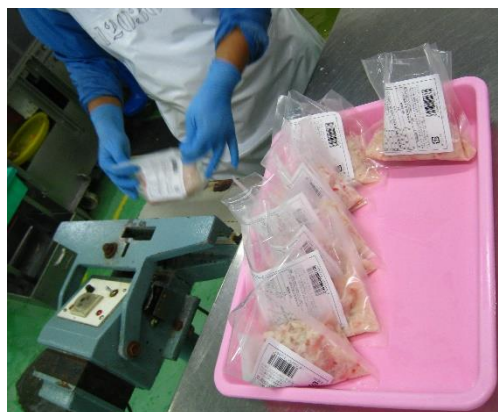
Figure 3-14: Packing (200g/bag) Process
