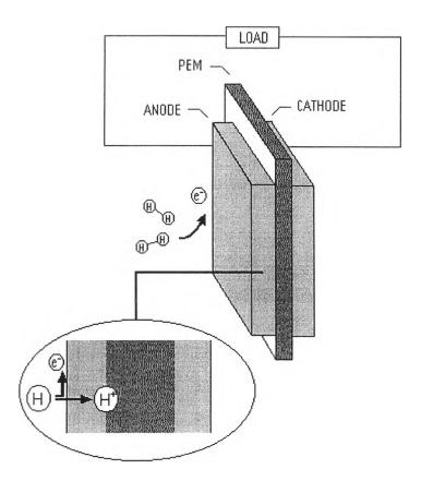
Figure 1.1 Operation of a polymer electrolyte fuel cell (PEFC).
