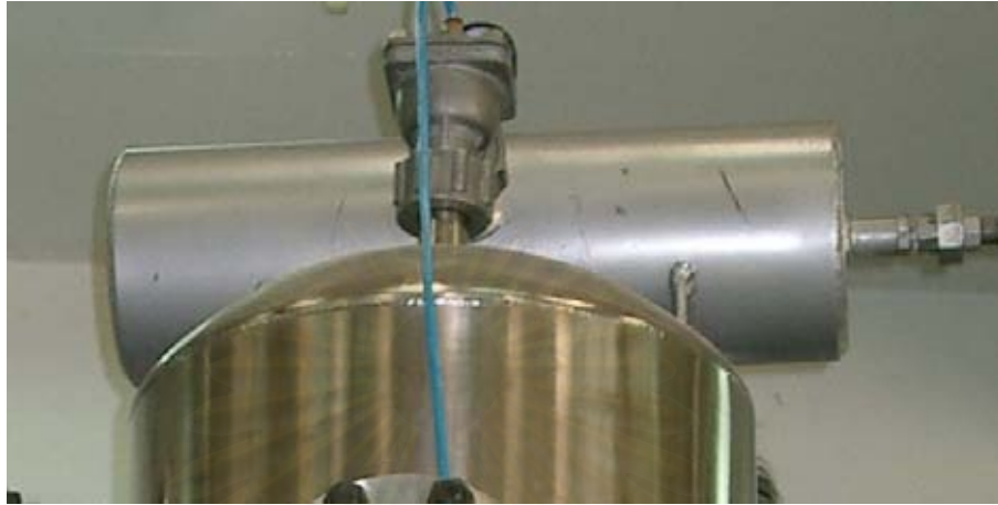
Figure 4.8 Pulse Air Tank
